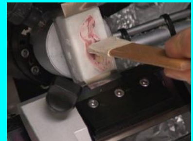
Fig. 2. Adhere the Cryofilm to the surface.
